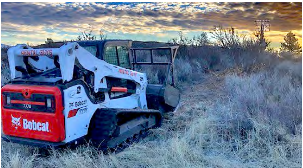
PSREC reduces wildfire risk by using Bobcat forestry cutters to clear right-of-way areas near utility poles.
