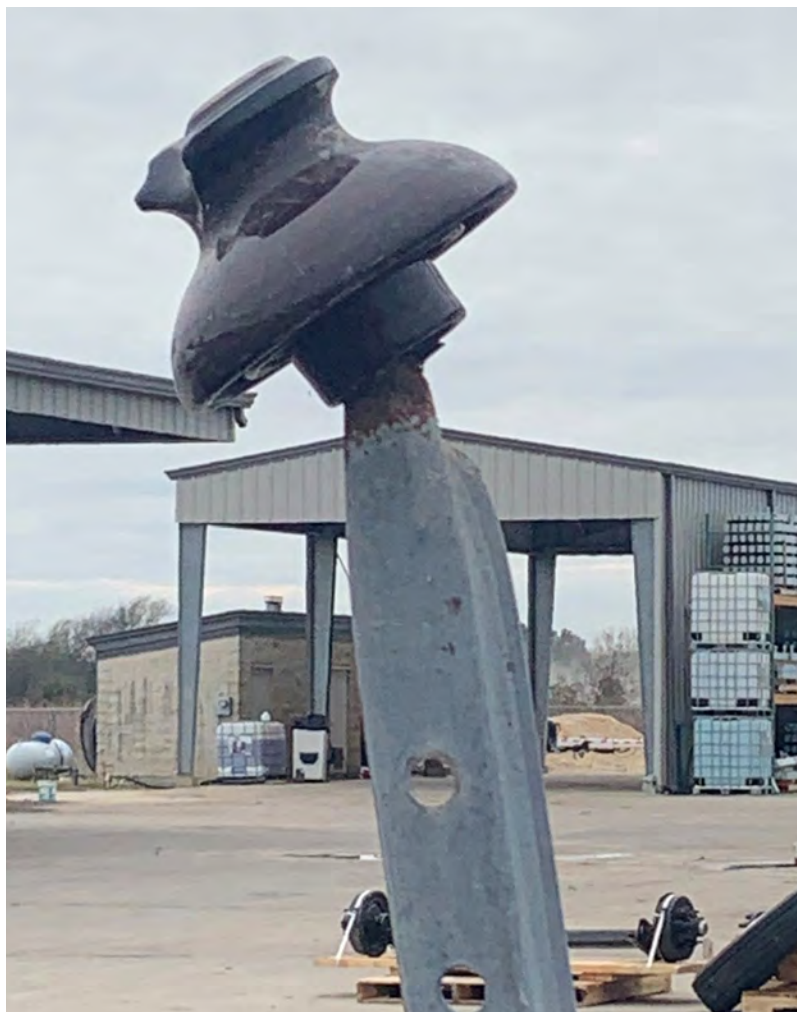
JEC uses fiberglass pole-top pin insulators to extend the life of its poles.
