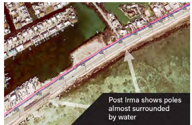
Beach erosion from Hurricane Irma prompted FKEC to relocate 37 transmission poles along Sea Oats Beach to the other side of U.S. Highway 1.
