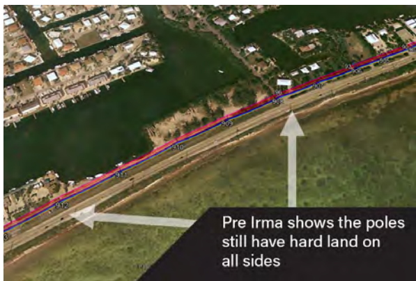
Beach erosion from Hurricane Irma prompted FKEC to relocate 37 transmission poles along Sea Oats Beach to the other side of U.S. Highway 1.
